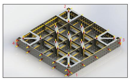
Follow this pattern when welding to slots together, Less is more when welding this table together, the more welding means more heat & higher chances or warping the table surface.
