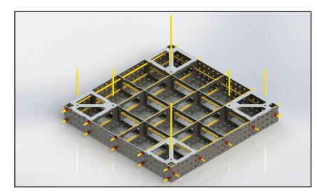
Insert the threaded rods into the table in both holes of the leg plates and make sure they line up with the corresponding holes on the table top.
