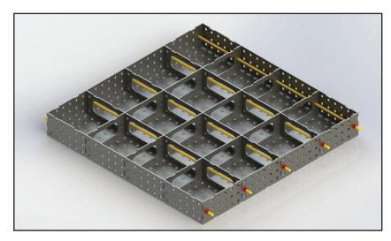
With the assistance of a second person begin to install 2 opposing table sides, use several pieces of the threaded rod to hold the opposing piece in place during the process. Add the next 2 oppsing sides, also using the threaded rod to hold the pices in place. Ensure the nuts on the threaded rod are only tightened just enough to hold the pieces in place & do not over tighten them.
